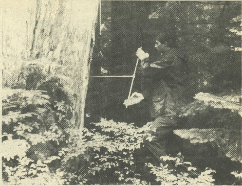
Taking a core sample with an increment borer from an ancient western red cedar in a fairway of the proposed Cypress Ridge golf course.
